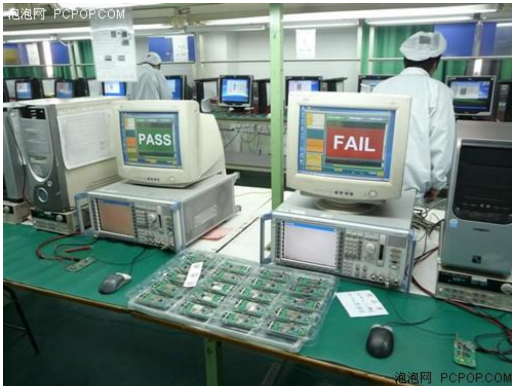
Figure 15. 测试台给手机主板加电测试 [13]
