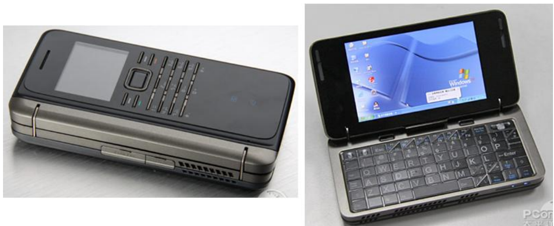
Figure 8.2 ViewSonic VCP08 is a combination of a XP Netbook, plus MTK feature phone.
