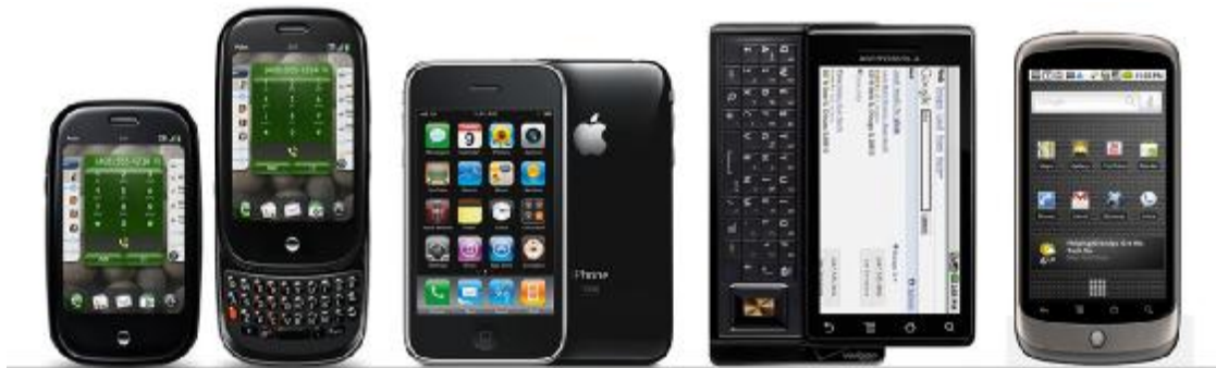
Figure 9.3 Palm Pre, iPhone 3GS, Moto Droid, Google Nexus One, all uses ARM Cortex-A8 CPU [10,11,12,13]。
