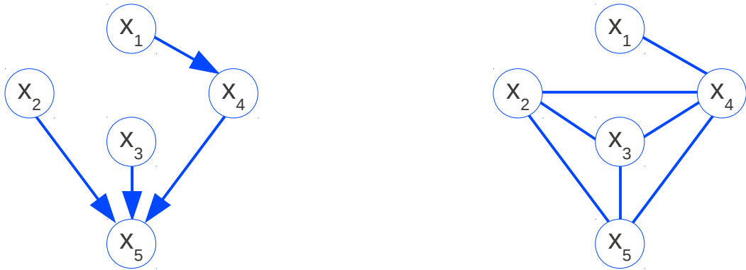
Figure 2.3: The moralization of the DAG on the left to obtain the moralized undirected graph on the right.
