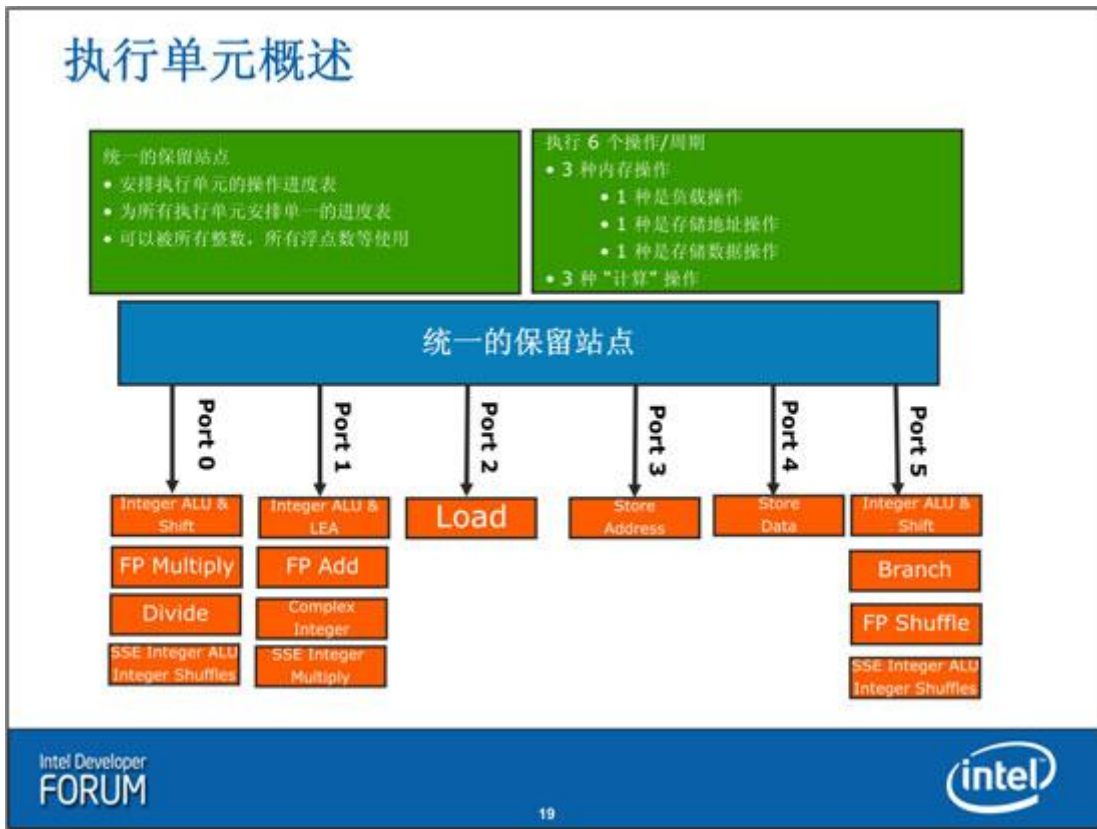
Nehalem:Superscale Execution Unit 超标量执行单元
