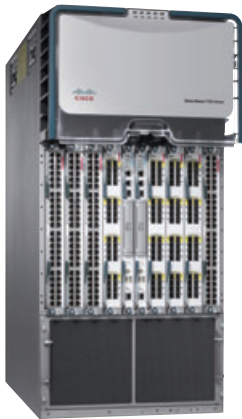
Cisco Nexus 7010 Data Center-Class Switch*
