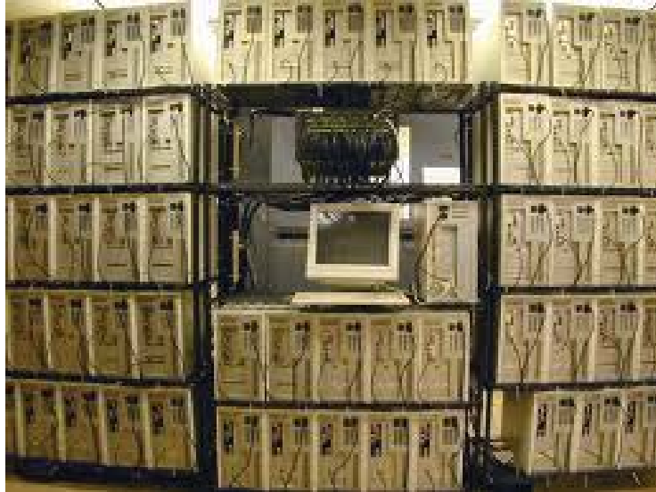
Figure 1.3: An 128 processor Beowulf cluster at NASA.
